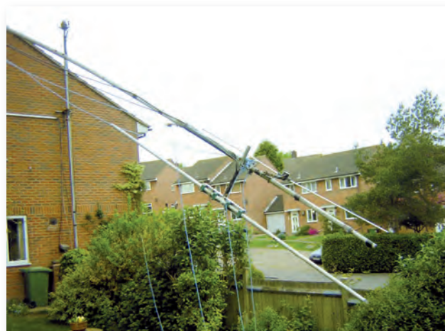
Fig. 3: The antenna, shown before erection to the working position, is 2.89m long and made from relatively large diameter tubing, which helps to increase the overall bandwidth.
