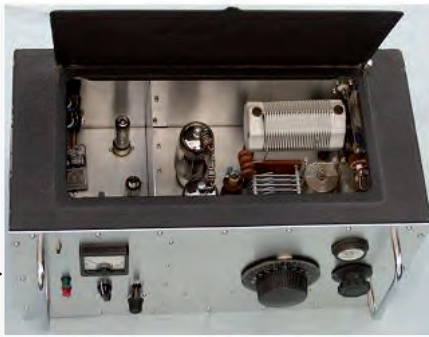
Fig. 2: Featured recently in The Signal was this 100W a.m. transmitter based on a pair of TT21 valve working in parallel.
