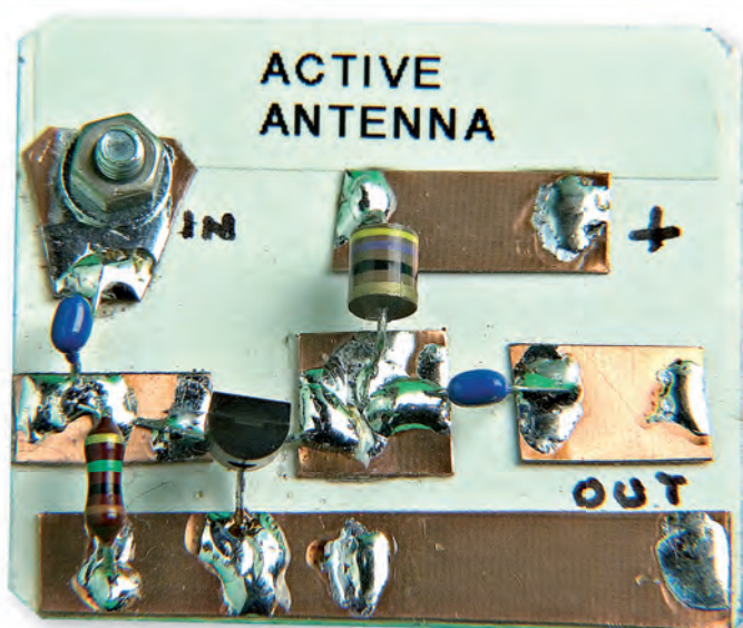
Fig. 2: The physical layout of the project of Fig. 1, created by George G3RJV sticking small pieces of p.c.b. material onto 2mm thick card.
